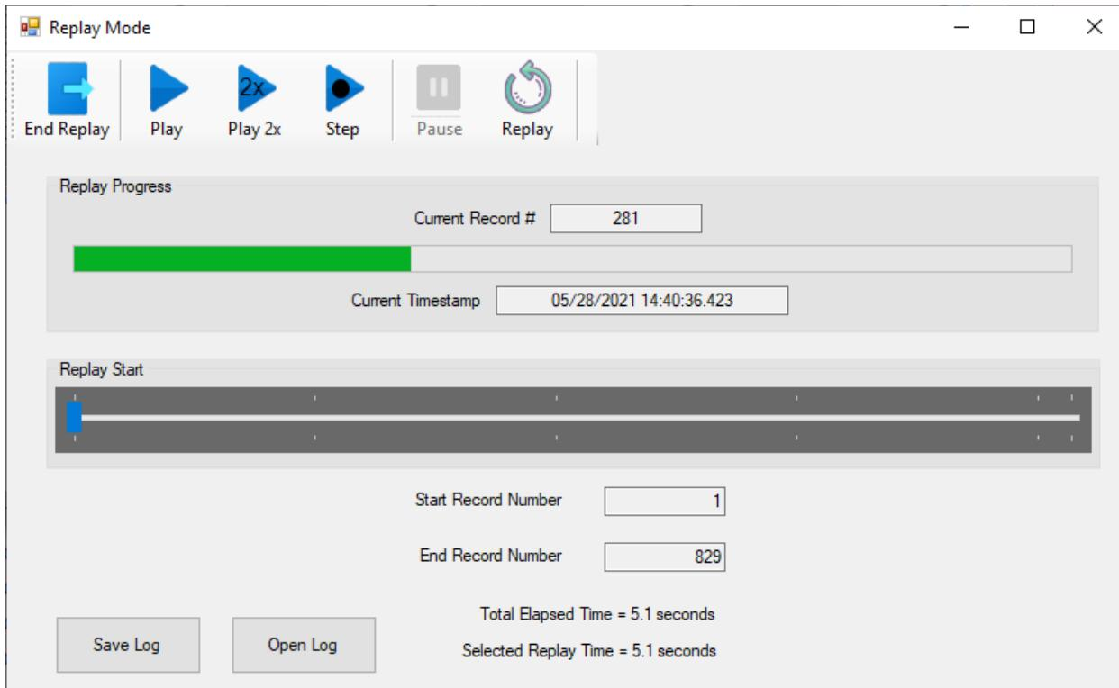
During the Replay Mode, the SIU Device View and Map View are not updated from the real time Controller SB#1 activity, but rather the replay of the records selected (Section 8.3.7). The SIU Device View panels are displayed with a blue border to indicate the Replay Mode is active.
