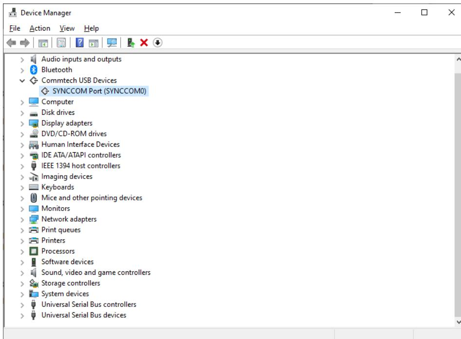
If this entry does not appear in the Device Manager, ensure that the USB cable is installed and that the HDLC Interface Module shows two green LEDs illuminated to the left of the DB-25 connector port. The top green LED indicates power to the module, and the bottom green LED indicates internal operation. The USB drivers may need to be reinstalled, see Section 2.4.
