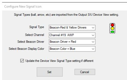
In the example shown above, the Beacon is driven from the Red output of channel 19. The Beacon display color is blue on the Map view, and the SIU Device view displays channel 19 driving Beacons from the Red and Yellow outputs.
