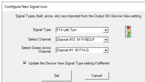
The Signal Type can be modified from the default selection provided by the Device View SIU channel panel if desired. Use the Signal Type pull-down box to select a different signal face. If the Device View SIU panel signal type should be updated to match this new selection ensure that the *Update the Device View Signal Type setting if different* checkbox is checked before clicking the Set button.
