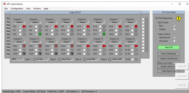
When linked to an Output SIU-2218, the colored signal indicators display that an output to the SIU is active. The associated checkbox can be checked to manually force the output to the active state when the Output Control radio button labeled *SIU Direct* is selected. See Section 4.3.3.3.
