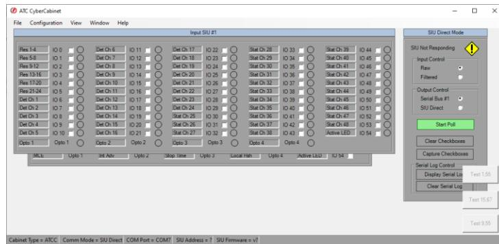
When linked to an Input SIU-2218, the blue circular indicators display that an input to the SIU is active. The associated checkbox can be checked to manually force the input to the active state when the *Output Control* radio button labeled *SIU Direct* is selected. See Section 4.3.3.3.
