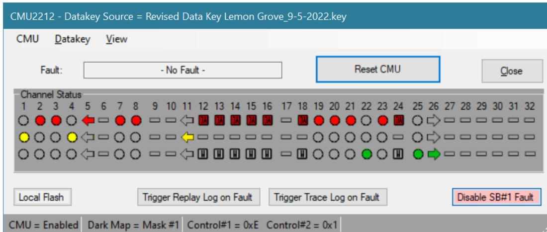
This CMU emulation provides a secondary benefit of validating the programming of the target intersection CMU Datakey configuration. The CMU configuration parameters can be read from an EDI *MonitorKey*® formatted disk file, or directly using the EDI *MonitorKey*® Programmer device.
