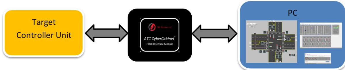
The *ATC CyberCabinet* software emulates the functionality of the ATCC Cabinet Monitor Unit (CMU) and input/output Serial Interface Units (SIU). Up to seven SIUs are supported, two Output SIUs and five Input SIUs. Several different configurations of ATC cabinets are supported (See Section 5.2.1):
