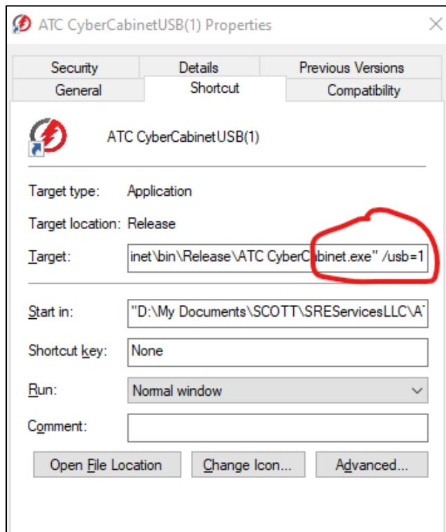
This shortcut process is only needed if additional HDLC Interface Modules are added. For a single instance, the program defaults to USB address 0.
